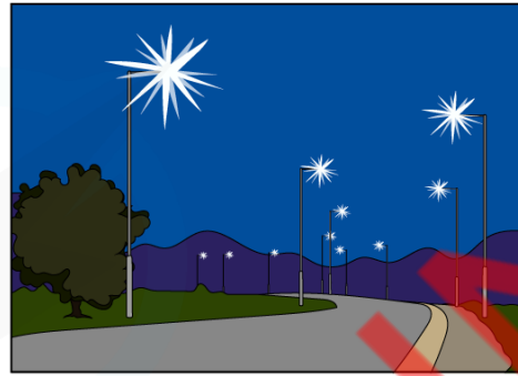
AT NIGHT, THERE IS LOW LIGHT INTENSITY → LDR SWITCHES LIGHTS ON
